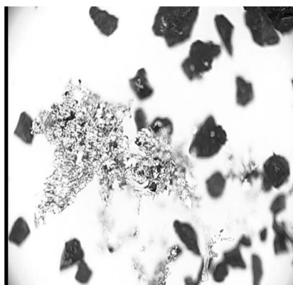
Figure 4. Gold particle formation by OW at high gold concentration ( \times 150 ).
